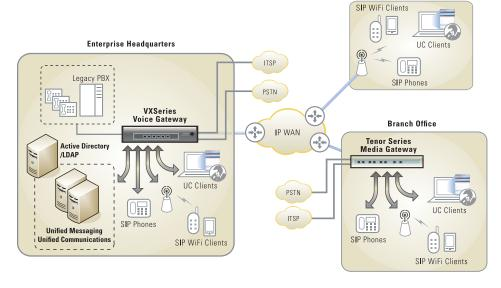
ENTERPRISE-CLASS INTEGRATION OF UNIFIED COMMUNICATIONS WITH TELECOM INFRASTRUCTURE: NET's VX Series and Tenor Series Media Gateways provide full connectivity between Unified Communica- tions and Telecom infrastructure. NET's portfolio meets the Media Gateway requirements for UC deployments for large to small enterprises for their headquarters and branch office locations.
